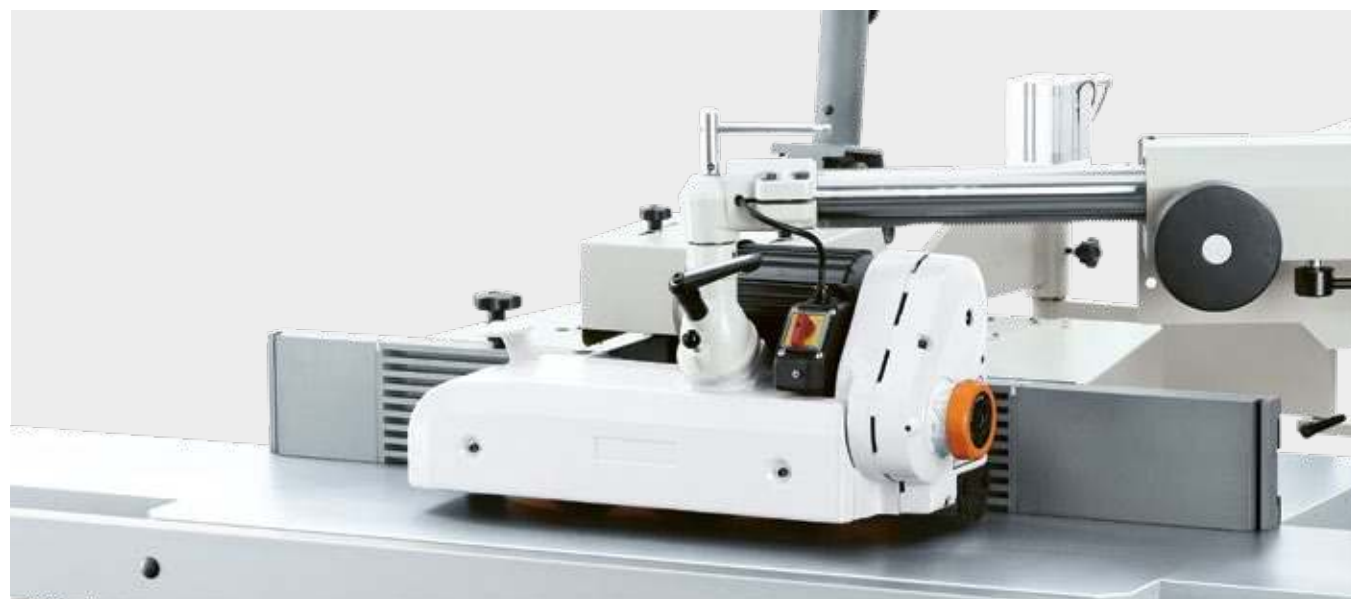
Posuw Variomatic 4N na suportie posuwu | T2923_400 + T2915
