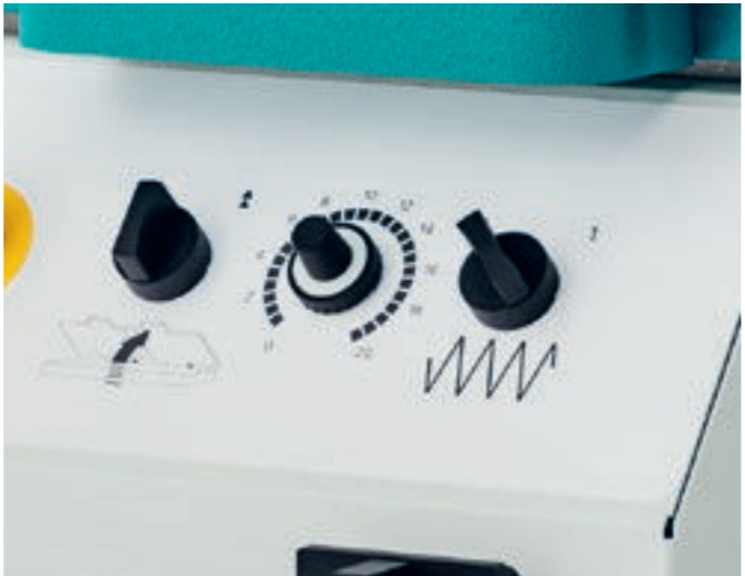
Continuously adjustable feed | T3221
