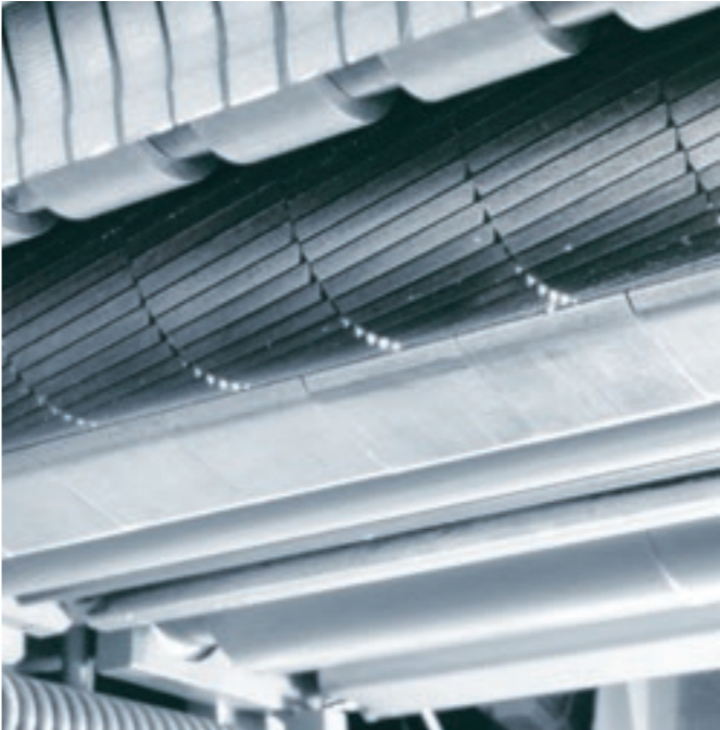
Steel jointed infeed roller | T4515
