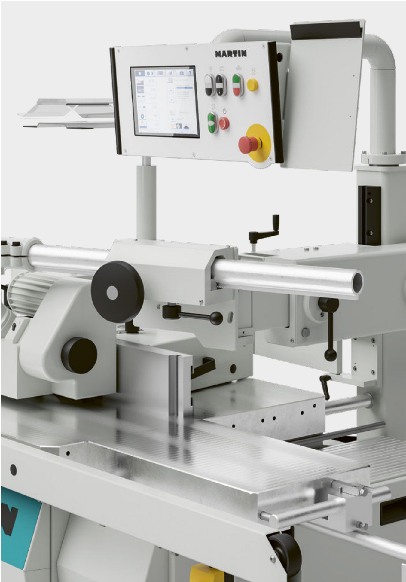
Control panel T12 | T27, ergonomic at eye level
